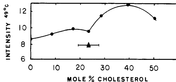
FIGURE 5: Relative intensity of DPH fluorescence (in arbitrary units) at 49 °C in DPPC-cholesterol multilamellar vesicles as a function of cholesterol content. A region of inflection occurs at about 22 mol % cholesterol, as indicated by a horizontal symbol (|—Δ—|).
